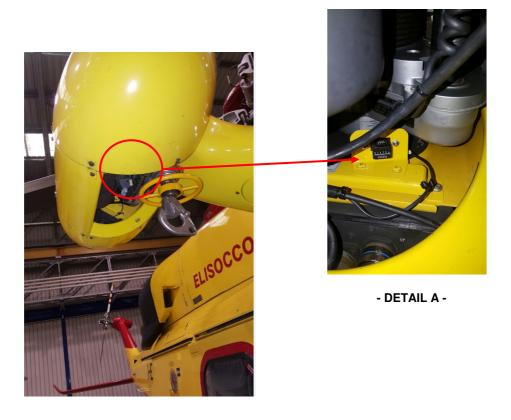
Figure 2 - Access and position of the Secondary Cycle Counter
