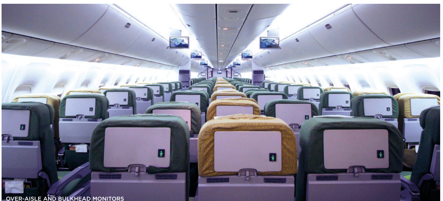
OVER-AISLE AND BULKHEAD MONITORS
